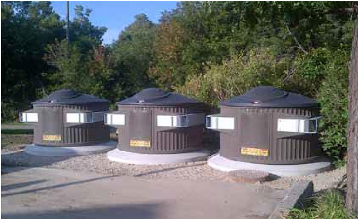
Second, the container holds more waste in a smaller footprint than a standard steel dumpster because much of the storage capacity is hidden underground. For example, 42% of the EnviroWirx's storage capacity is underground, which helps to disguise the actual mass of the container.
